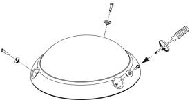
Tighten the 3 diffuser fixing screws + the screw covers on the diffuser using a suitable screwdriver and the **98000003** vandal-resistant bit.
