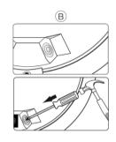
In order to ensure the luminaire is sealed, it is vital to use the cable grommets.
